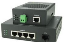
When you need to extend Ethernet services beyond the general IEEE 802.3 limits of 328ft / 100m in extreme temperatures, and new fiber cabling is cost prohibitive, Ethernet Extenders are the perfect solution. Perle Ethernet Extenders transparently extend up to four 10/100/1000 Ethernet connections across copper wiring. Use single twisted pair ( CAT5/6/7 ) or any existing copper wiring previously used in alarm circuits, E1/T1 circuits, RS-232, RS-422, RS-485, CCTV and CATV applications.
